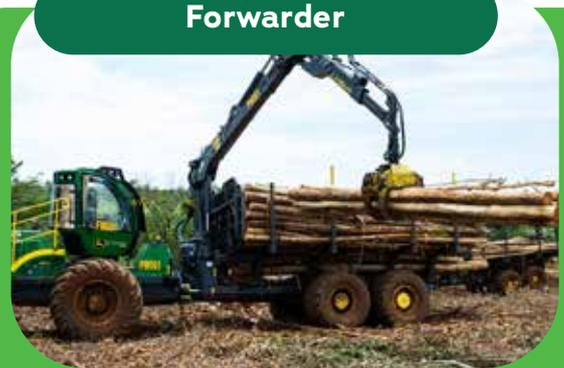
Forwarders convey processed wood logs from the site to the roadsides, where they are piled up for subsequent transportation to the industrial plant.
