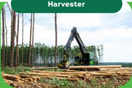
Tree felling, branch and twig removal, bark stripping, and cutting into specified lengths are carried out by harvesters. Log bundles are stored for subsequent transshipment, which usually takes place around 10 days after felling.
